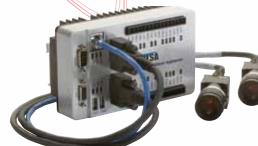
**Multi Point Inspection** - DALSA's Vision Appliances offer solutions for both single and multi point inspection. Packaged complete with application software, these systems comprise a centralized controller with expandable camera interfaces to deliver high performance processing with low deployment cost.
